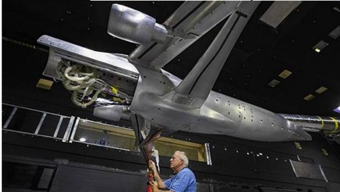
Researchers completed TTBW high-lift tests, including stability and control checks and ground-effects evaluations, in September at NASA Langley Research Center’s 14 X 22-ft. subsonic wind tunnel in Hampton, Virginia.
